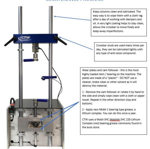
Inside the machine, there are industrial bearings that all have grease fittings that can be used along with a grease gun for lubricating. This does not need to be done but once every three years under normal operating of the machine.
